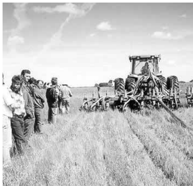
Low-disturbance injection into standing soil.
