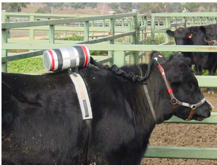
Figure 3. Steer fitted with methane collection apparatus. (From: Hegarty et al. 2007)
