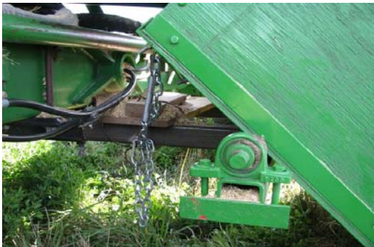
Photo 10: Chaff box hinge using a pillow block and bearing.
