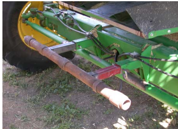
Photo 9: Chaff box hinge using 2 3/8 in. pipe and 2 7/8 in. collar.
