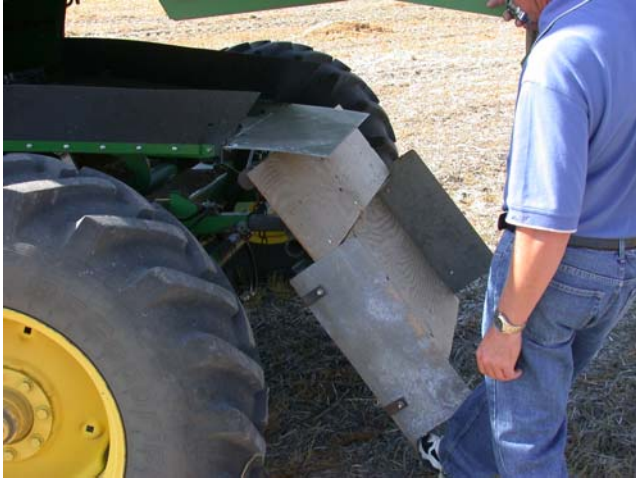
Photo 12: When tipped, the chaff box should be four to five in. off the ground.
